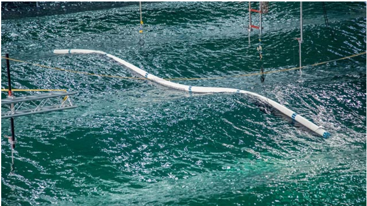
Hundreds of scale model tests were conducted throughout the years to refine the design and predict the behavior and performance of the system
