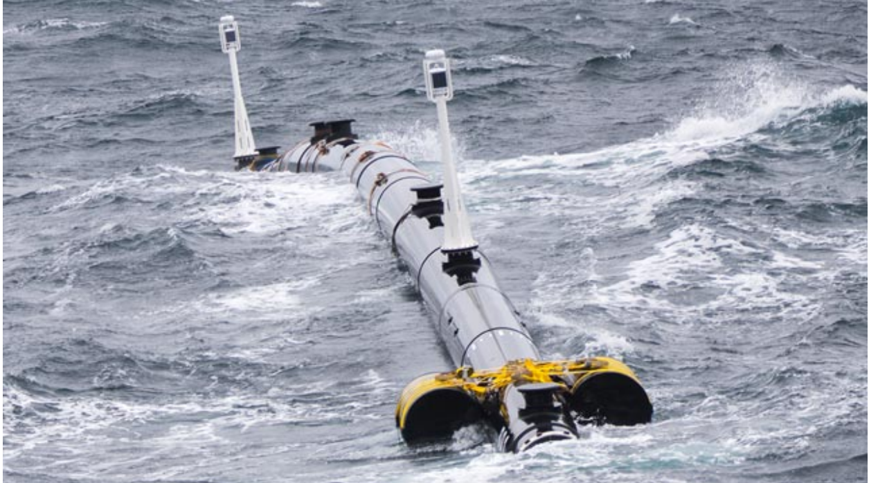
In May 2018, a 120-meter section of the system successfully passed a tow test in the Pacific Ocean, being subjected to waves of up to 5 meters.
