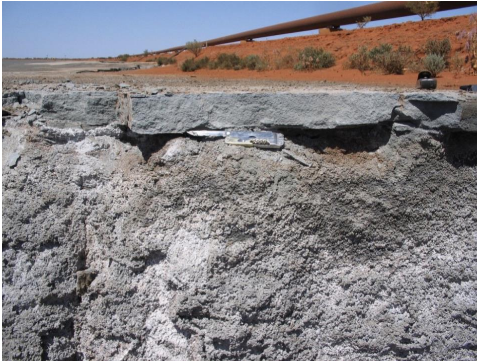
Cementation of tailings originally deposited as water-sand slurry. LOCATION: Mt. Keith Nickel Mine, WA, Australia. Greg Dipple
