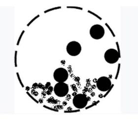
A **ball mill** or **roller mill** is a type of grinder used to grind or blend materials for use in paints, pyrotechnics, ceramics, and selective laser sintering. It works on the principle of impact and attrition: size reduction is done by impact as the balls drop from near the top of the shell. The process of grinding is called **comminution**.
