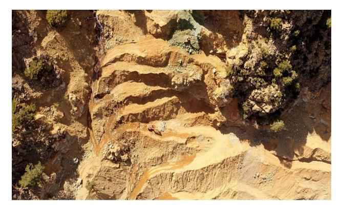
The above shows the world's largest active olivine quarry, **Gusdal Pit**, in Norway. No chemicals are needed to extract the rock, nothing is underground, the process is not mining, it is surface extraction. This raises the possibility of purchasing olivine on site, ensuring it is finely ground, and immediately distributing it in the ocean.
