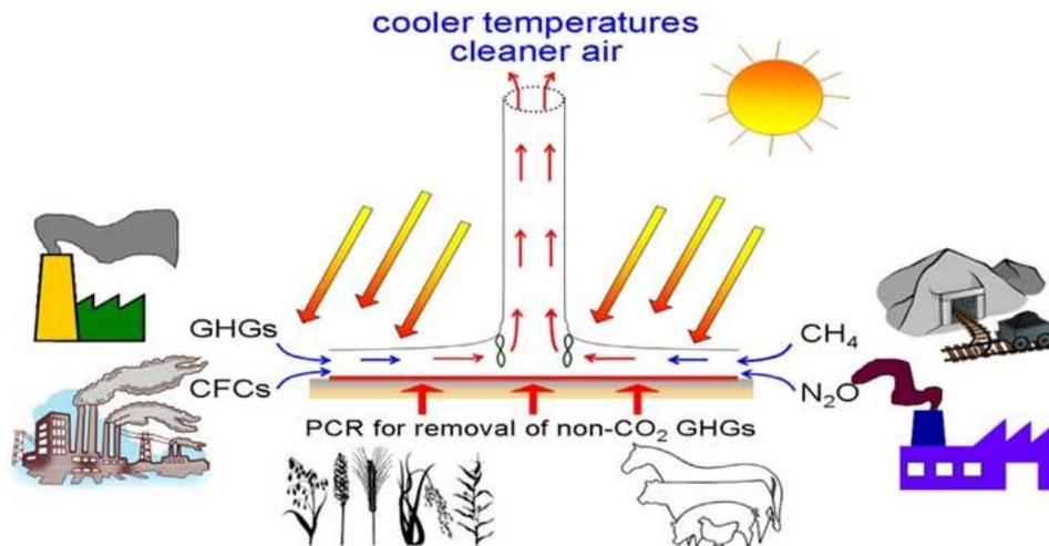
The SCPP is an established concept that generates electricity in a solar updraft tower incorporating axial-flow turbines. Hot air is supplied to the tower by a large solar hot air collector. A conventional **SCPP-PCR** is composed of 4 principal components:
